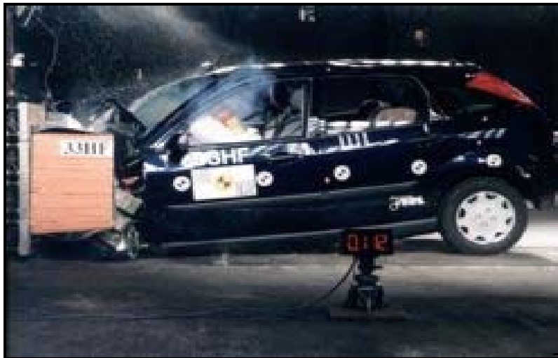
Figure 10. Euro NCAP LHD Reference vehicle at maximum intrusion
